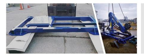
Crane Base made from 80mm x 160mm x 6.3mm Box section with a 25mm thick mounting plate for the crane to sit on. All holes drilled and extra holes strategically drilled to allow for galvanising to be carried out without compromising on structural integrity.
