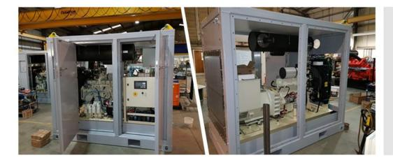
Generator housing containers built in accordance with and certified to DNV 2.7.1 standard. Bespoke build to house generators and with exhaust mount brackets and access panels, doors, removable ends and bund wall.
