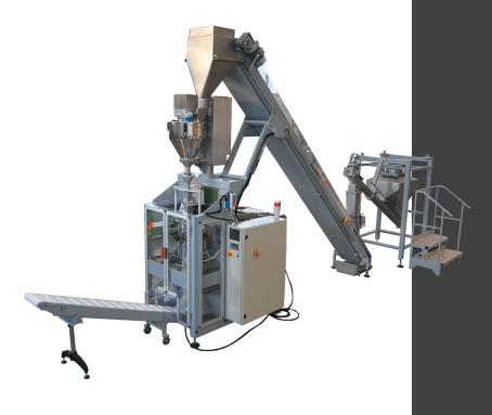
The FPK 42 is the smallest packaging system in the form fill & seal series. It is ideal for those looking to pack 1 - 5Kg bags. Together with a multi-head weigher, the system is capable of achieving up to 60 bags a minute, depending on the product type.
