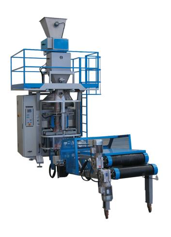
The FPK 46 provides the perfect solution for those looking to bag Animal feeds, cat litter or wood pellets. It has the ability to reach a throughput of 16 bags a minute, depending on product type and bag size. The FPK 46 is one of the most popular Form, Fill & Seal machines available, due to its versatility to lend itself to many products along with its robust mechanical components.
