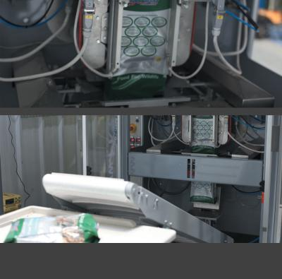
The FPK 44 is one of the most popular Form Fill & Seal vertical bagging systems. It proves to be extremely versatile to handle most applications. Previous installations include packaging lines for wood pellets, animal feeds, rock salt, wet sand and other aggregates.
