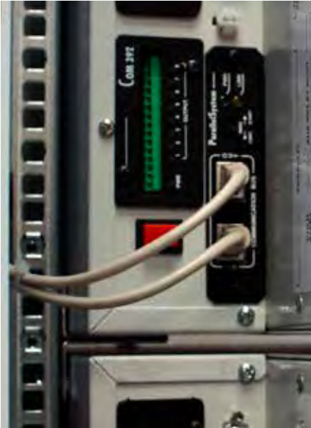
Parallel configuration and programmable relay contacts board
