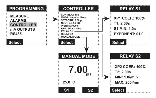
The controller output (Y) activates the limit switch relays. The Y value may correspond to a control by impulse of a control by frequency. The Y value is determined by the parameters below:
