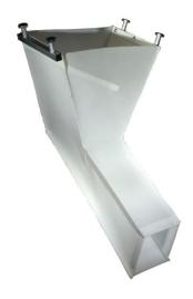
The collecting funnel ATB-S with diagonal runout is mounted under the tool of an injection moulding machine via strong permanent magnets. It safely collects the moulded parts after demoulding and transfers them onto a conveyor belt or into a container next to the machine. The funnel is movable and follows the tool. Optional equipment such as a baffler or a removable base ensures damage-free collection and waste reduction of the moulded parts.
