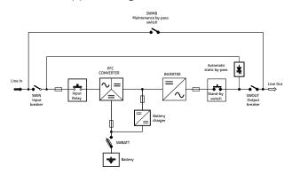
Figure 6 – Diagram of UPS with separate battery charger
