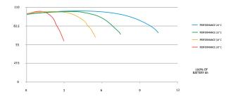
Figure 3 – Graph plotted from temperature multiplier table showing battery performance at constant temperatures
