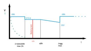
Figure 8 – Cyclic charging voltage plot
