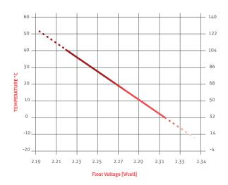
Figure 4 – Recommended cell charging voltage against temperature
