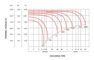
Figure 9 – Battery voltage discharge curve at varyin discharge rates
