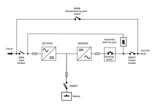
Figure 5 – Diagram of UPS with combined rectifier and battery charger
