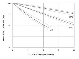
Figure 10 – Battery self discharge at varying temperatures
