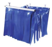
The collecting funnel ATB-L with lamellas is mounted under the tool of an injection moulding machine via strong permanent magnets. It safely catches the moulded parts after demoulding and passes them onto a conveyor belt or into a container below the machine. The funnel is moveable and follows the tool. Cooling or tempering hoses can be passed through the lamellas easily, without new complex placement of the hoses.
