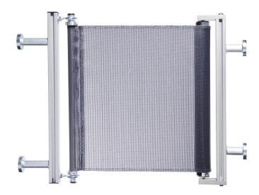
The side protection curtain RS is attached to the side of the tool or the clamping plates of an injection molding machine via strong permanent magnets. It catches moulded parts after demoulding to prevent the parts from contamination, reduces waste and keeps the environment of the machine clean. The materials used are view permeable and partially FDA approved.
