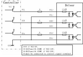
Figure 3: Connection to PNP signal (common-cathode)
