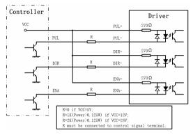
Figure 2: Connections to open-collector signal (common-anode)
