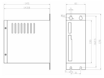
Figure 1: Mechanical specifications
