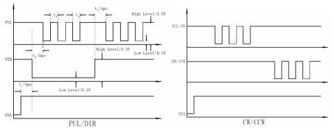
Figure 11: Sequence chart of control signals
