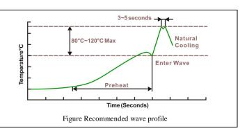
The upper side temperature of the board should not exceed +150°C.
