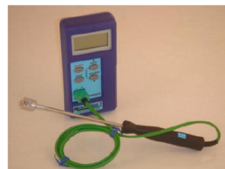
Thermometer and s/s band surface probe to check jaw temperatures.
