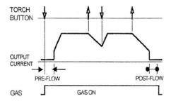
When the trigger mode is in the 4 step position the following sequence will occur
