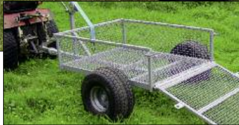
Fitted with optional loading ramp and winch
