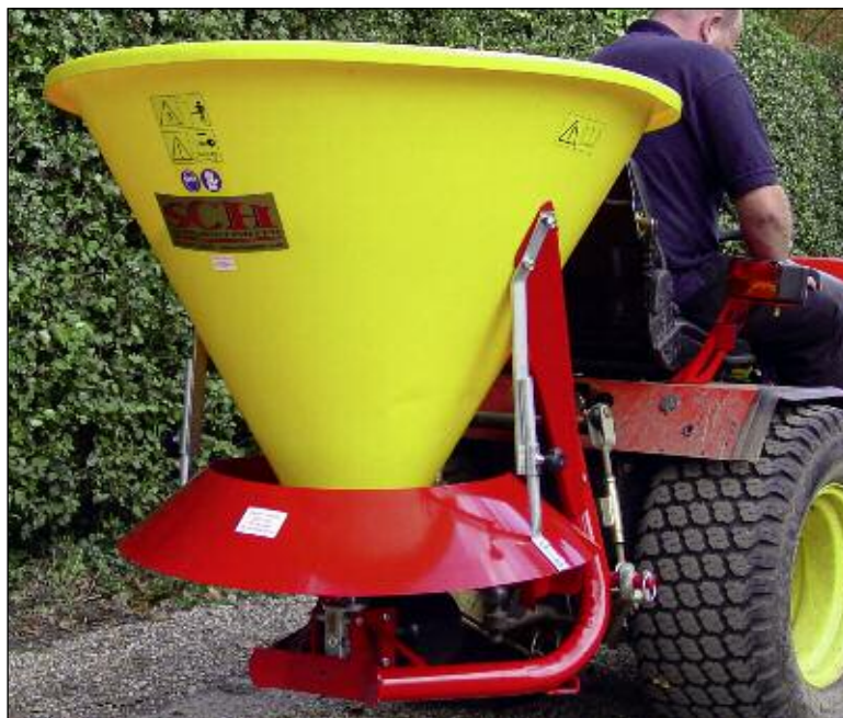
This shows the unit fitted with an optional deflector guard
