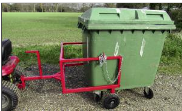
Shown with optional jockey wheel and winch. The trailer illustrated is for 'off road' or 'slow tow' use only.
