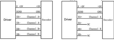
Figure 5: The DSB810A supplies the differential encoder directly
