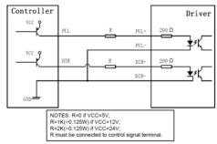
Figure 3: Connections to PNP signal (common-cathode)
