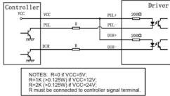
Figure 2: Connections to open-collector control signal (common-anode)
