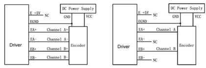
Figure 7: Using external DC power supply to supply the differential encoder
