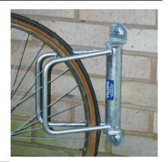
The simplest cycle holder, a familiar sight throughout the UK, allows the tyre of the bicycle to be supported. The stand is fixed to a suitable wall and can be spaced at no less than 610mm between holders for cost effective cycle parking. The Model R is available in either 90° or 45° versions which allow for cycles to be parked either head-on or angled.
