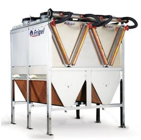
**Summit TPC Premium Adiabatic Coolers** do not create external aerosols but utilise an internationally patented chamber keeping the adiabatic process within the unit. This system also keeps the coil blocks dry eliminating scaling and avoiding the risk of proliferation of bacteria such as legionella.
