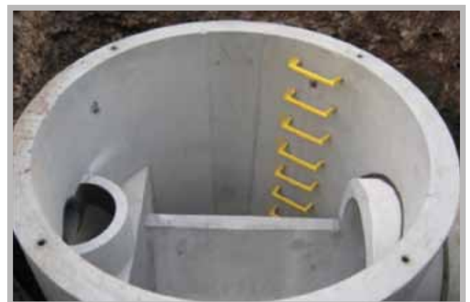
2100mm diameter wide wall manhole complete with pre-fitted ovoid butt and channel plus internal back-drop junction
