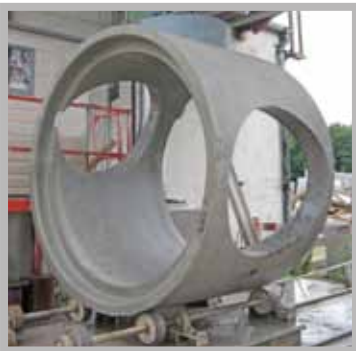
1800mm sealed manhole being cored for a 900mm internal diameter pipe
