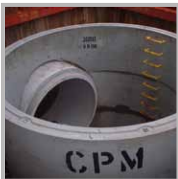
3000mm wide wall sectional chamber, 1800mm inlet and 1050mm outlet, pre-fitted Hydro-Brake® and penstock.
