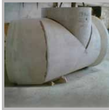
1200mm side entry being manufactured
