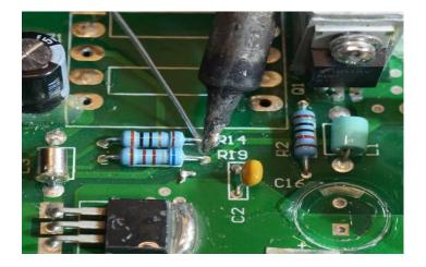
Fothershield distribute MG Chemicals superior Lead-Free flux cored solder wires, pastes and flux. The solders are made from virgin metals, have higher melting temperatures and wet metal surfaces more slowly. Joints will look different as the surfaces are not as reflective as tin-lead joints.
