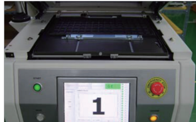
View of a pallet which has moved up to the upper change rack from the STF-100N model after all the materials in it were exhausted.
