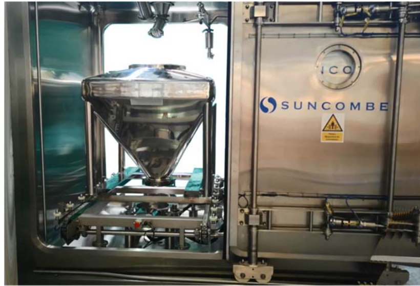
IBCWashBooth™ with Conveyor Feed, Passthrough Automatic Doors, Automatic Lid Removal, Automatic Spray Device Insertion, Split Containment Valve Opening, and Drying.
