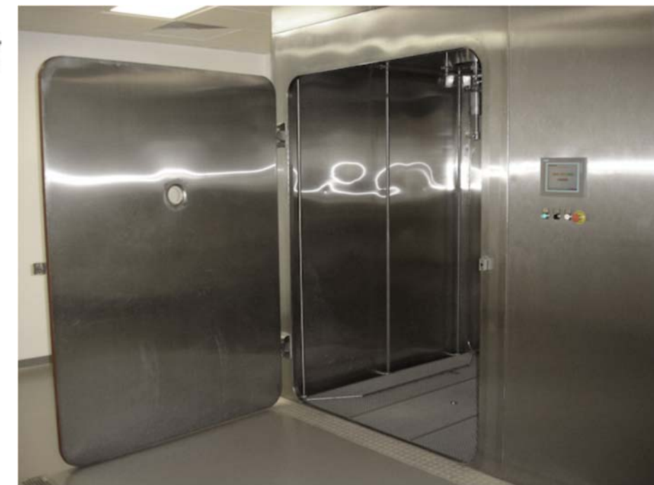
Installed IBCWashBooth™ configured with remote equipment
