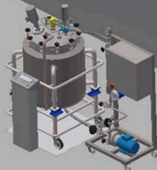
Mobile Process Vessel with integrated WIP System for semi-automatic Wash In Place
