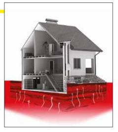
treatment areas, mining operations and peat bogs. Methane can migrate through subsoil and through cracks and fissures into buildings and structures. A build-up of methane to hazardous levels will cause harm to health and compromise safety.
