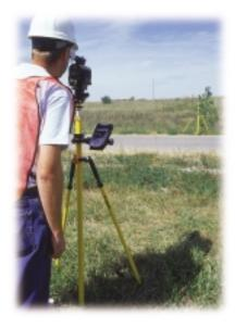
A One-Person, Line-Of-Sight Operation, the Terrain-Mapping system uses a reflective laser to direct a beam to a stationary prism, which reflects the beam back to the laser providing height and distance readings. The program can provide a range of distance up to 1200 feet (366 m) without moving the prism.
