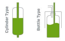
The Swagelok grab sampling systems provide solutions to satisfy gas and liquid non-slurry sampling service in a consistent, reliable package. Two system types allow for capture into one of two types of containers — pressure-containing metal cylinders as found in the Grab Sample Module (GSM) or non-pressure-containing glass or polyethylene bottles as found in the Liquid Only Sampling Module (GSL).
