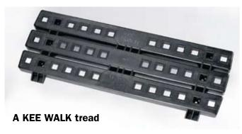
Manufactured in high grade nylon incorporating raised roughened sections, the treads are developed to comply with EN 516 (Prefabricated Accessories for Roofing – Installations for roof access – Walkways, treads and steps), exceeding the deflection criteria and slip resistance requirements of the standard.
