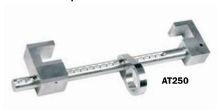
A temporary lightweight aluminium anchor point for use with steel beams. Tested to EN795 Class B, adjustable for beams between 95mm and 400mm flange.
