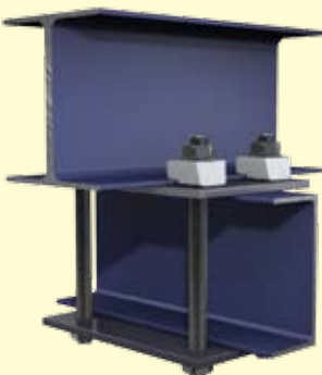
Channel section below I-Section at 90 degrees
