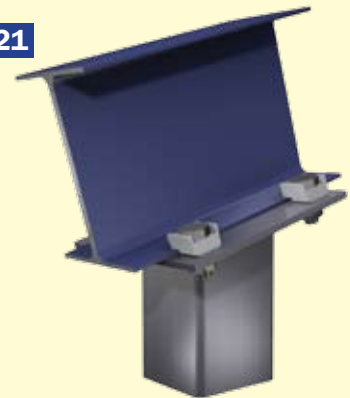
Column end plate to sloping I-Section
