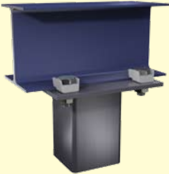
Column end plate to I-Section
