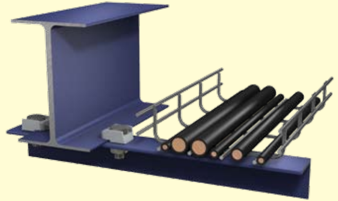
Cantilevered angle support for running cable tray
