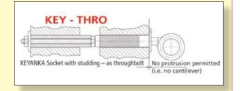
**KEY-THRO** Standard **KEYANKA** socket with additional M12 threaded extender. For use as through bolt fixing (e.g. in cavity walls). NO cantilever permitted.
