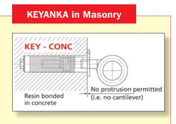
**KEY-CONC** Standard **KEYANKA** socket suitable for resin bonding into minimum 150mm thick concrete ONLY. NO cantilever permitted.
