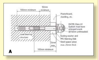
We also offer **Cantilever Anchor Devices** for use in dry lined walls or in conjunction with plasterboard, cladding etc. Where the distance from the face of the load bearing structure to the collar of the eyebolt does not exceed 25mm, a **spacer sleeve** may be placed under the eyebolt collar to provide the necessary support (Fig. A).
