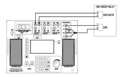
Figure 3.1 Connection for 120V relay
