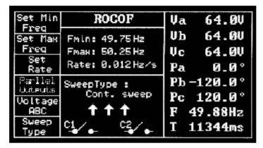
Figure 2.1 DVS3 ROCOF mode
