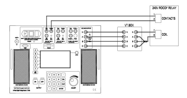
Figure 3.2 Connection for 240V relay
