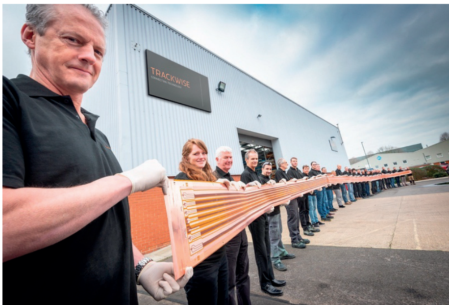
Figure 3: A 26m-long, multi-layer flexible printed circuit for a UAV
