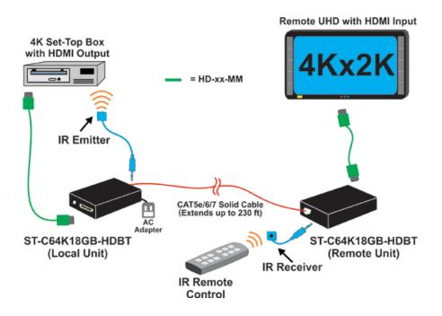
The ST-C64K18GB-HDBT transmits uncompressed digital Ultra-HD HDMI 4Kx2K 60Hz 4:4:4 signal, IR, RS232, Ethernet, and power up to 230 feet over a single CAT5e/6/7 solid cable using HDBase-T technology.
