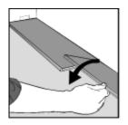
3. Fold the board down with a single action movement to locate the header joint **ensuring the joint "clicks" and locks.**
