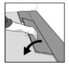
8. Place the board tight to the short end of the previous board and fold down in a single action movement **ensuring the short joint "clicks" and locks correctly**.
