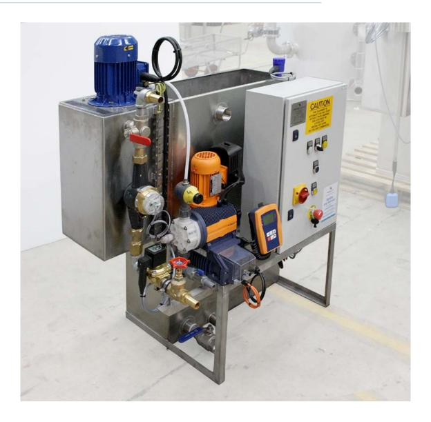
The EMU – CTS is supplied as a skid unit. It comprises a polymer feed pump and the electrical control panel mounted on a stainless steel frame, a flash mixing tank with agitator, a 200 litre tank, integral storage with level probes, polymer inlet pipework, three way valve on the water inlet, a solenoid valve and pulsing water meter on the water inlet. Also supplied with an IBC, Sotz connector and 3m of chemical delivery hose. The unit is supplied pre—wired ready for operation.
