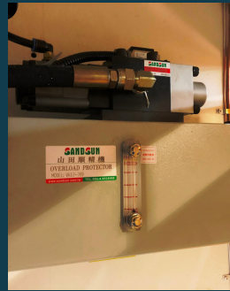
HYDRAULIC OVERLOAD PROTECTION
