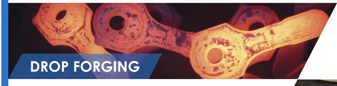
DROP FORGED COMPONENTS FROM 25GRM UP TO 75KG NET WEIGHT
