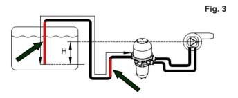
In order to avoid possible problems, each burner or appliance should have its own separate suction line. Also, we recommend one Tigerloop® Bio for each burner. Remember to use nozzle capacity (fuel consumption) to calculate the dimension of the suction line.
