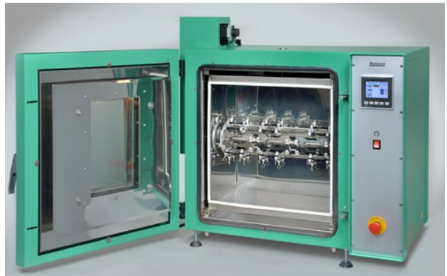
Cabinet ageing oven EB 26 with a carousel, which rotates during ageing.
