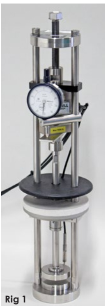
Rig 1 is arranged for testing in compression according to ISO 3384.
