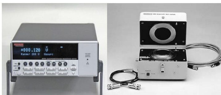
EE 04-II Volume Resistivity tester for determination of volume and surface resistivity on insulated materials includes a voltage instrument and a resistivity test fixture.
