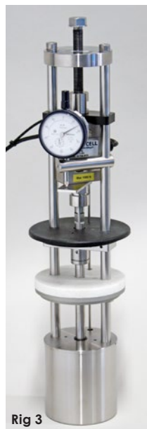
Rig 3 is arranged for testing in liquid according to ISO 3384.
