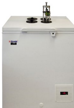
Combined low temperature instrument with a Gehman Tester selected, on the adjustable table ET 01.08.
