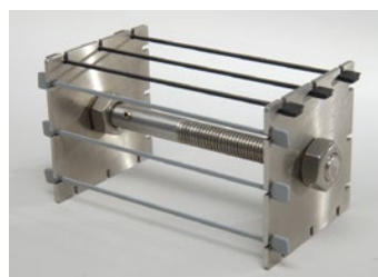
Tension Set Rig, EV 04.
