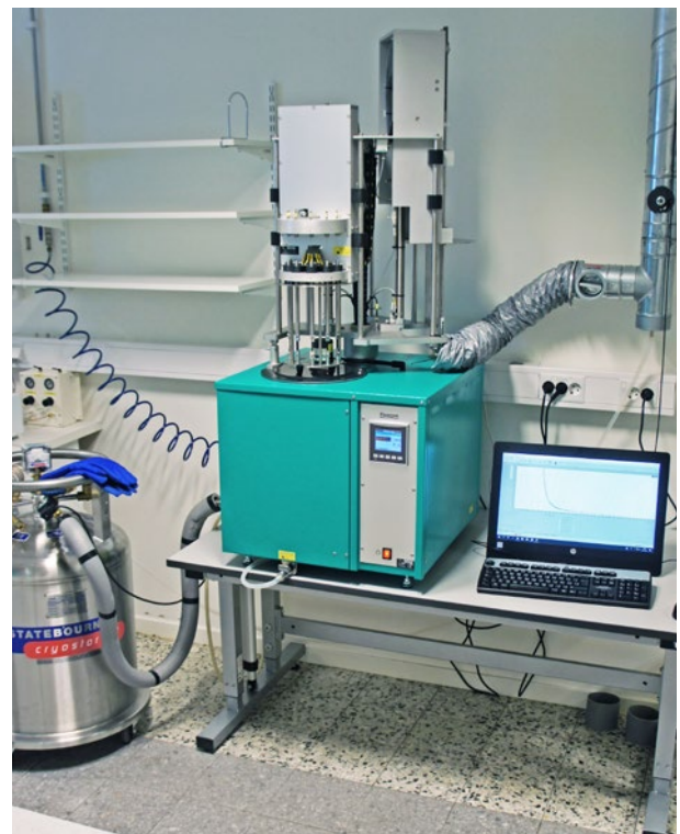
Combined low temperature instrument with a Gehman Tester selected, on the adjustable table ET 01.08.
