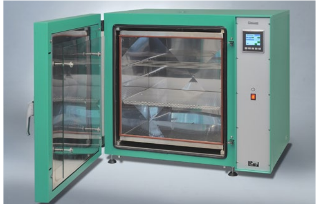
Cabinet ageing oven EB 10-II with a factory set throttle to give a fixed air exchange rate of 7 or 14 changes per hour.
