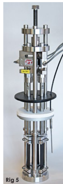
Rig 5 is our latest addition for testing relaxation in tension, a triple rig where you can perform a triple test in the same rig.
