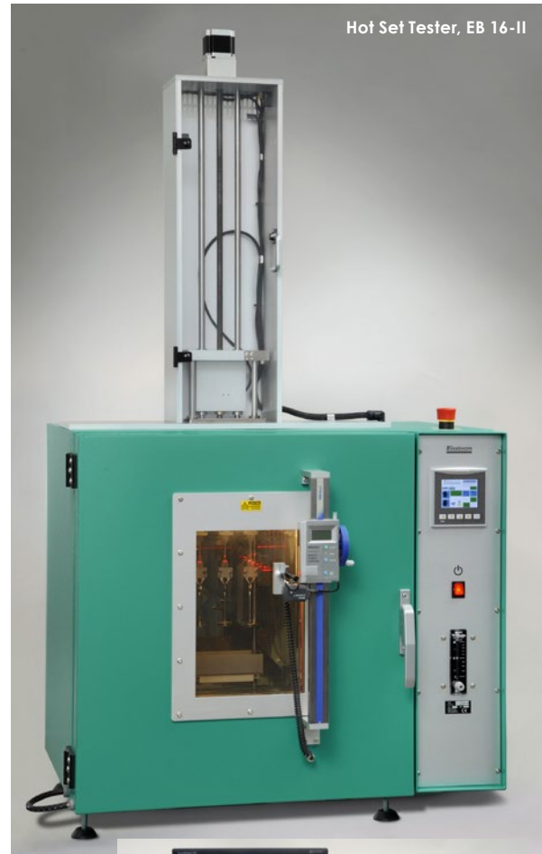
A computer, a digital caliper as well as clamps and weights for 8 samples are included with the EB 16-II.
