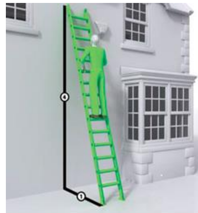
Figure 1 Ladder showing the correct 1 in 4 angle (means of securing omitted for clarity)
