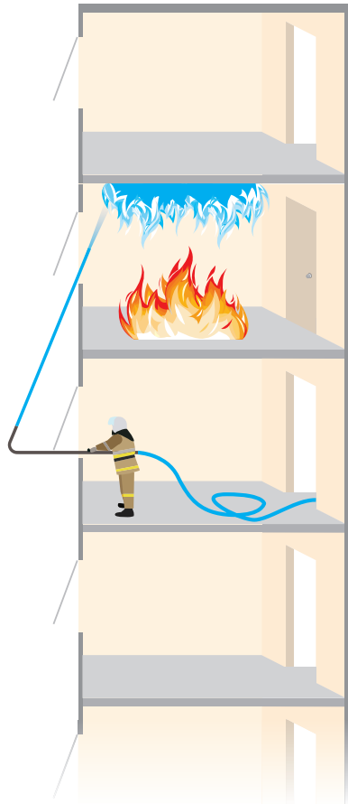
The Floor Below Nozzle (above, left) is specifically designed to be long enough to protrude out of a lower window, where the angled barrel is raked upwards, firing a solid jet of water through the upper window, hitting the ceiling and rapidly gas cooling prior to fire crew entry.
