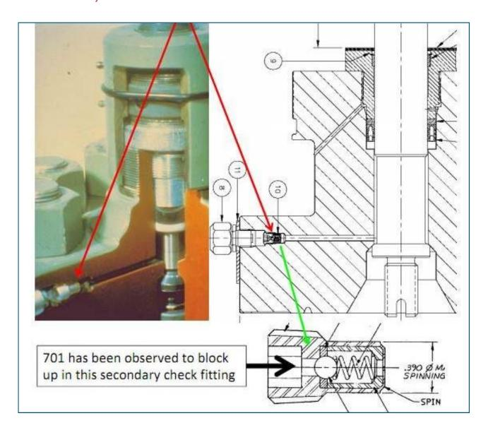
Prior to injecting 701, the operator should identify the exact make, model and pressure rating of the gate valve, and confirm the arrangement of the sealant injection fitting (s) in the valves bonnet. If there is any doubt, it is recommended that test pumping 701 through a spare fitting, attached to the pump delivery hose end should be conducted before injection into the valve.
