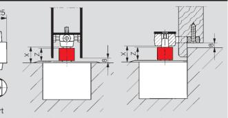
**NOTE:** Closer and bottom strap must be installed per fixing instructions for door clearances shown to be valid. Closers with extended spindle inserts are used with thresholds, carpeted floors, terazzo pans or in cases where more clearance between door and floor is required. Surface finish: Zinc plaed.
