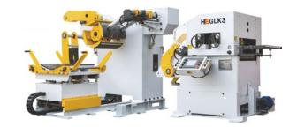
Founded in 2002 in Shenzhen China, Hong-Er Machine Equipment Co Ltd manufactures high quality coil handling and press feeding systems including decoilers, straighteners, feeders and compact coil feeding lines. CE Approved with English operator manual and electrical schematics.
