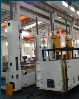
TIE ROD FRAME CONSTRUCTION
