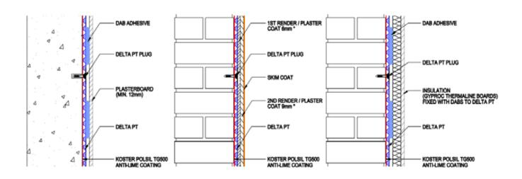
\*RENDER: 1:1:5 CEMENT: LIME: SAND PLASTER: TARMAC WHITEWALL (FOR OTHER PROPRIETARY PLASTERS PLEASE CONTACT DELTA TECHNICAL)
