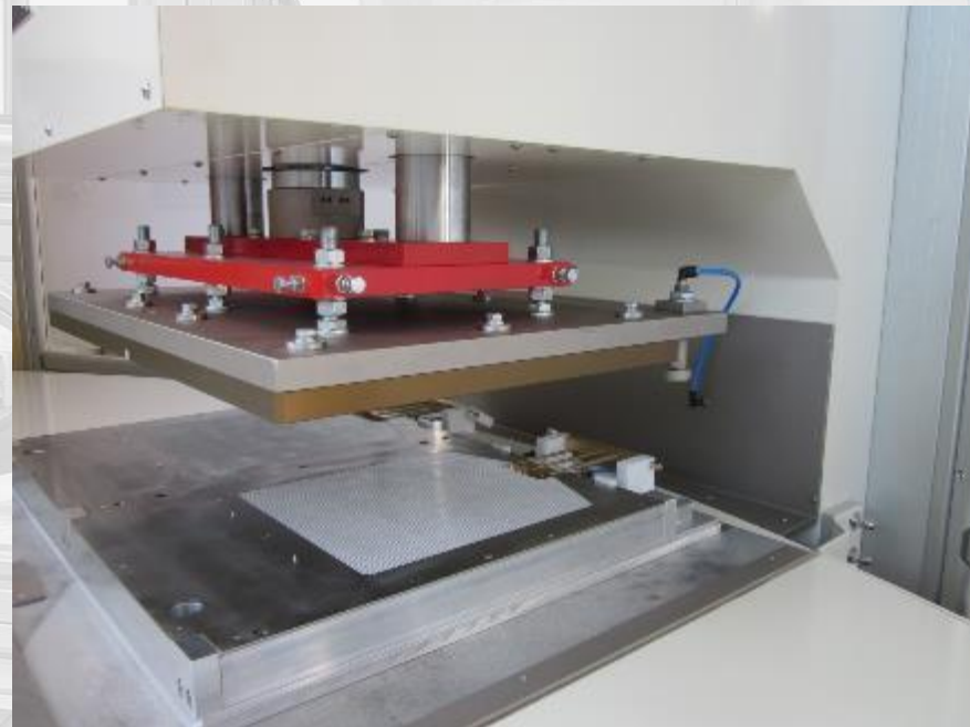
In line bags leakage control station
