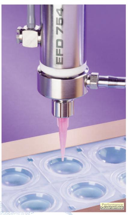
The 754V-SS aseptic dispense valve system accurately controls the application of most low to medium viscosity fluids. The seal-less design incorporates an inert PTFE diaphragm that isolates the actuator from the valve.
