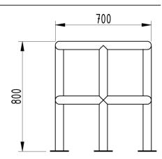
Functional and robust in design, AUTOPA's range of column protectors are designed to protect corners, columns, and other vulnerable pillars from vehicle damage in a busy industrial environment. Our Column Protectors are manufactured from mild steel and galvanised to ensure their longevity. Suitable for both internal and external use.
