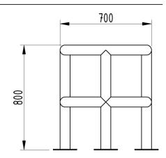
Functional and robust in design, AUTOPA's range of column protectors are designed to protect corners, columns, and other vulnerable pillars from vehicle damage in a busy industrial environment. Our Column Protectors are manufactured from mild steel and galvanised to ensure their longevity. Suitable for both internal and external use.
