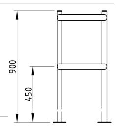
Functional and robust in design, AUTOPA's range of column protectors are designed to protect corners, columns, and other vulnerable pillars from vehicle damage in a busy industrial environment. Our Column Protectors are manufactured from mild steel and galvanised to ensure their longevity. Suitable for both internal and external use.
