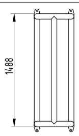
Functional and robust in design, AUTOPA's range of vertical column protectors are designed to protect pipes and other vulnerable pillars from vehicle damage in a busy industrial environment. Manufactured from mild steel and galvanised to ensure their longevity. Suitable for both internal and external use.
