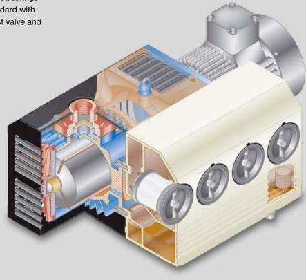
Once through oil lubricated rotary vane vacuum pumps
